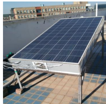
Fig.( b) Testing platform of the PV/T component
