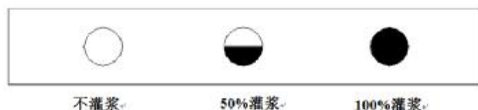
Fig. 2. Conditions for grouting of pre-stressed pipe
