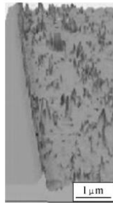
Figure 2. The etching topography of the gas flow at 72sccm
