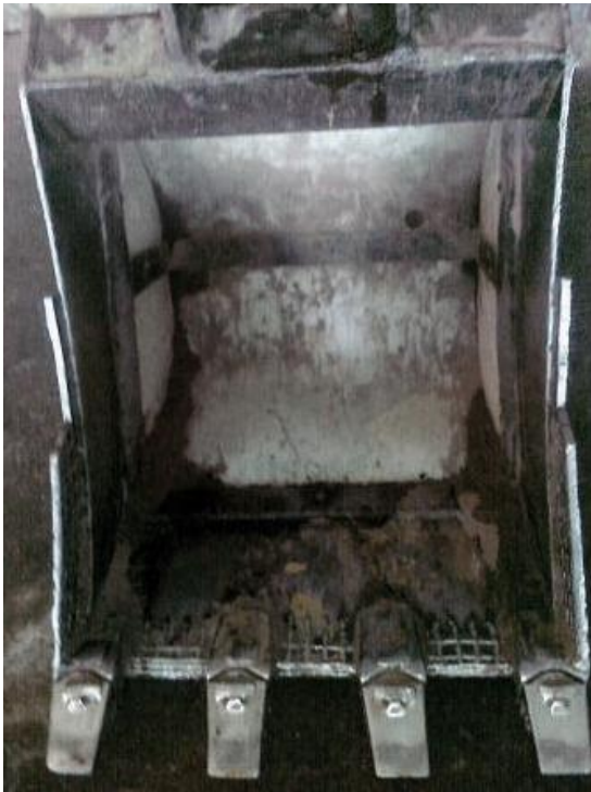
Fig. 10. EK-18 excavator bucket lined with anti-adhesive sheets
