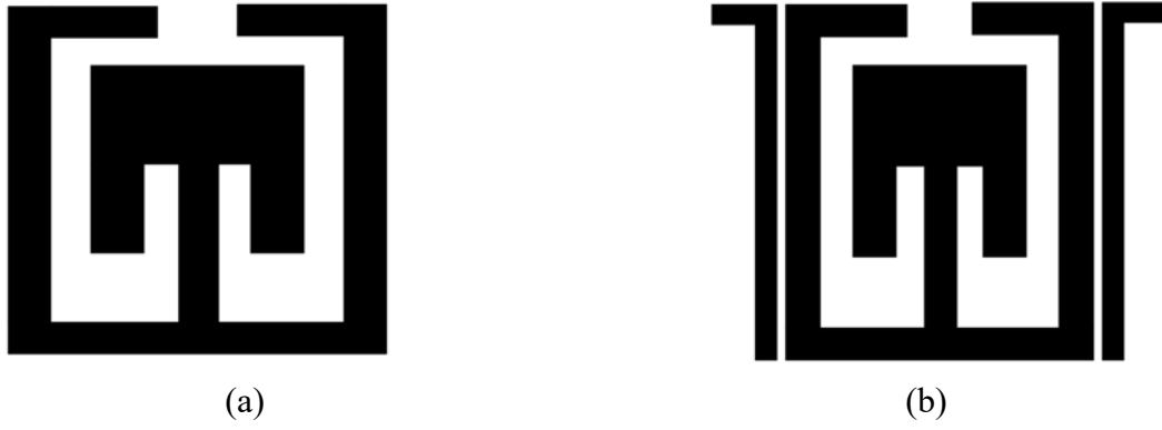
Fig 1. Dual-mode open-loop resonator and filter (a) Resonator, (b) Filter
