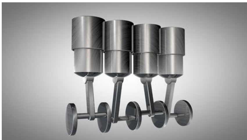
Figure 3. Reciprocating Motion Diagram of Cylinder Piston of Internal Combustion Engine
