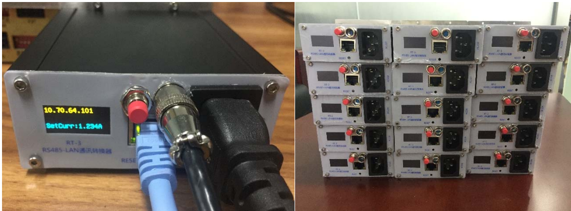
Fig 2.RS485-LAN converter Real photos
