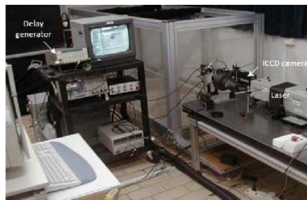
Fig. 5 Active laser imaging experiment system
