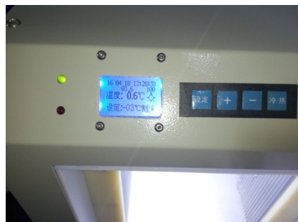
Figure 10. information diagram of the basic operating state of the temperature control box
