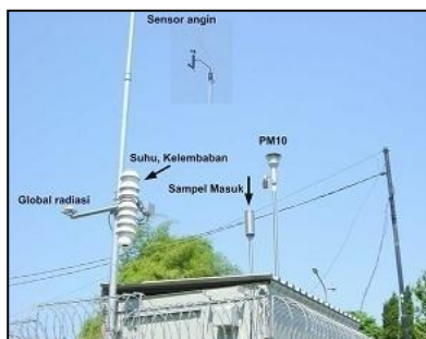
Fig 3. Sensor device of the air quality monitoring station (Surabaya city government, 2010)
