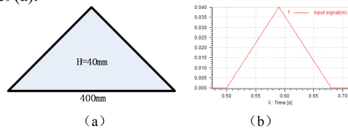
Figure 8. the standard pulse road block and the input signal in AMESIM
