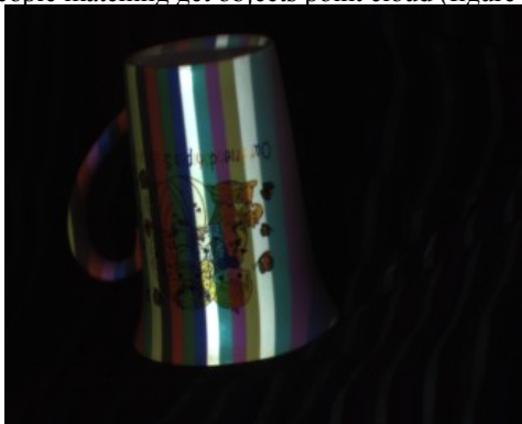
Figure 4. bits binary-coded color pattern projection
