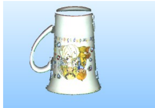
Figure 6. The points cloud with stereo matching
