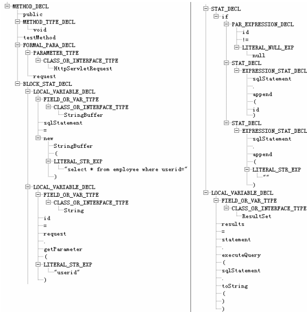
Figure2. Abstract syntax tree according to source code
