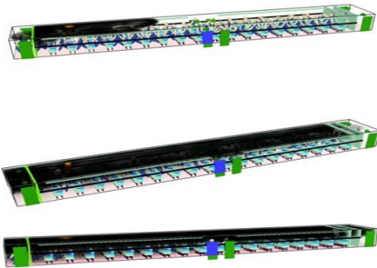
Figure 8. The spread of the smoke in the cabin
