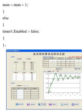
Figure 6 relief valve dynamic property curve diagram
