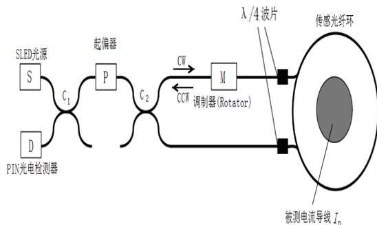
Figure 1. Schematic of the passive AFOCT.
