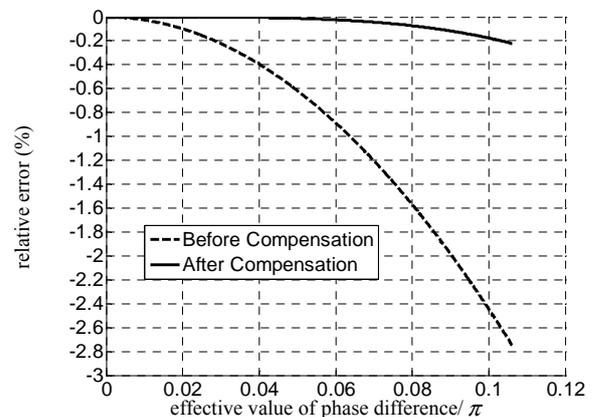
Figure 2 Relative error analysis of the passive AFOCT
