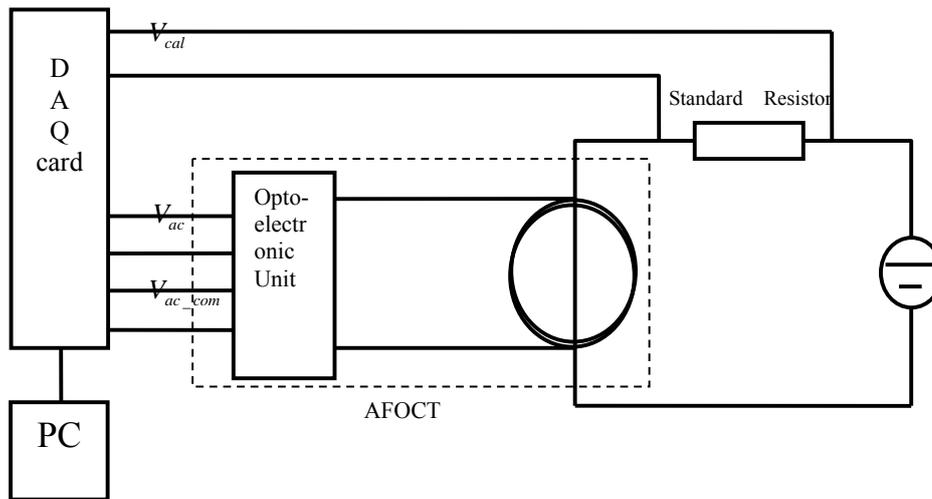
Figure 3 Experimental setup to test the scale factor
