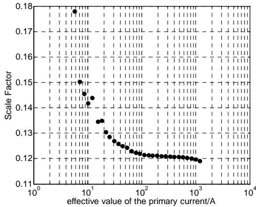
Figure 4 Scale factors of different primary current
