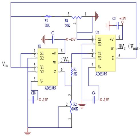
Figure 5 Schematic of the compensate circuit
