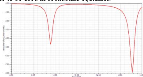
Fig.1 Two resonating frequencies caused by one resonator
