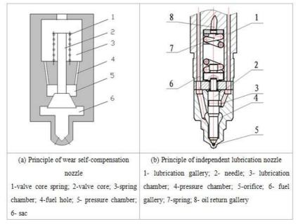
Fig. 2 principles of the new types of nozzles
