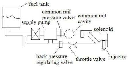
Fig. 1 dimethyl ether fuel injection system with throttle valve
