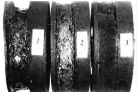
Fig. 8. Samples of Maslyanits: D (C-1) (1), KS-2 (2) and KSC (3), tested under dynamic loading ( p = 1254 N)
