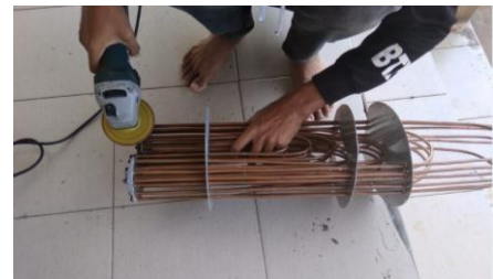
Fig. 10. Building Process of U-Tube Model
