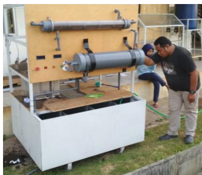
Fig. 11. Installing the shell and U tube
