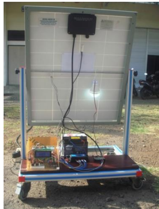
Fig.4 SHS prototype with the installed DAQ device
