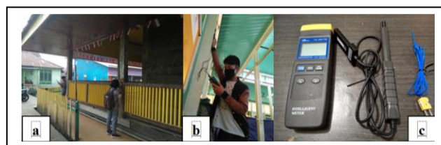
Fig. 10. The measurement of (a) Exterior Columns (b) Interior Columns (c) RH-T Digital Instrument
