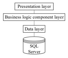
Figure 1 system logic architecture diagram
