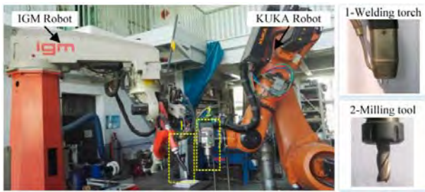
FIGURE I. TWO-ROBOT COOPERATIVE PLATFORM OF HYBRID MANUFACTURE
