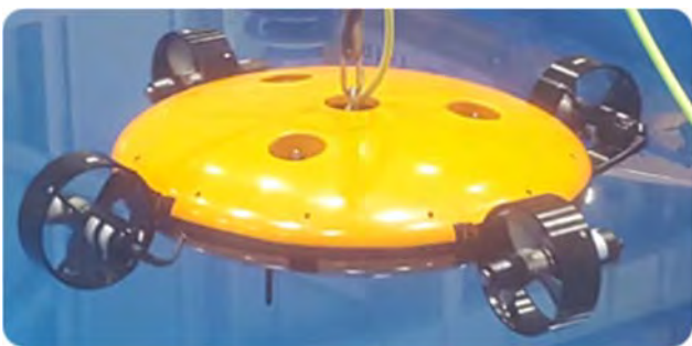
FIGURE 1. UUV PLATFORM WITH THE FLATTEND ELLIPSOIDAL EXTERIOR.
