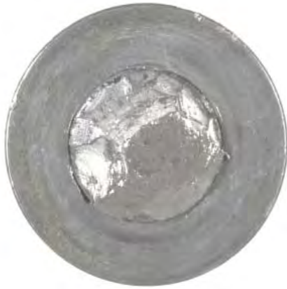
FIGURE II. MORPHOLOGY OF THE FRACTURE OF LEFT BOLT
