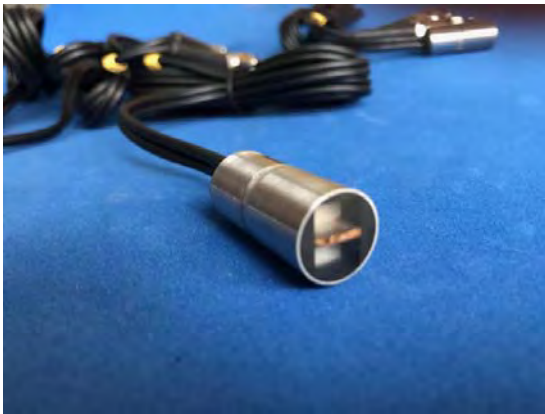
FIGURE IV. SCHEMATIC DIAGRAM OF TWIN - CRYSTAL PROBE AND TWIN - CRYSTAL PROBE
