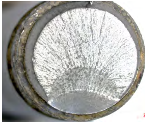
FIGURE III. MACROSCOPIC MORPHOLOGY OF INTERMEDIATE BOLT (HEREINAFTER REFERRED TO AS BOLT NO.2)
