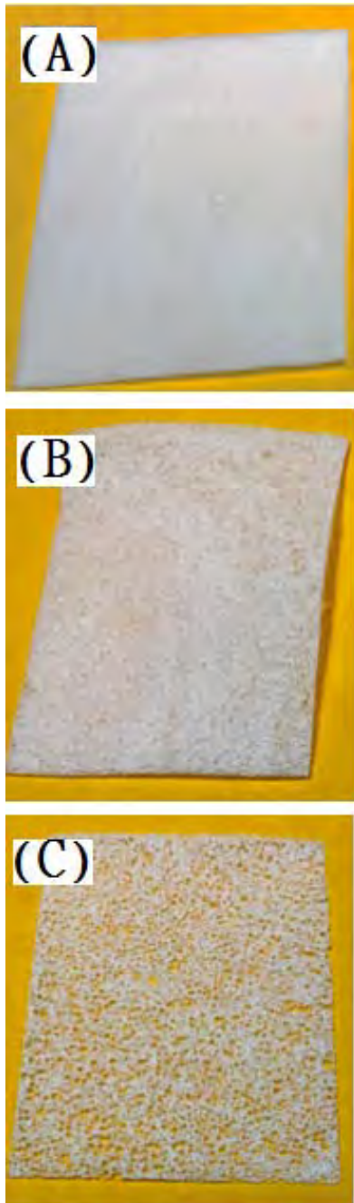
FIGURE I. PHOTOS OF THE RESULTING EXTRA THIN FOAM DRESSINGS FOR NPWT(A)PVAETF1, (B) PVAETF2, AND (C) PVAETF3
