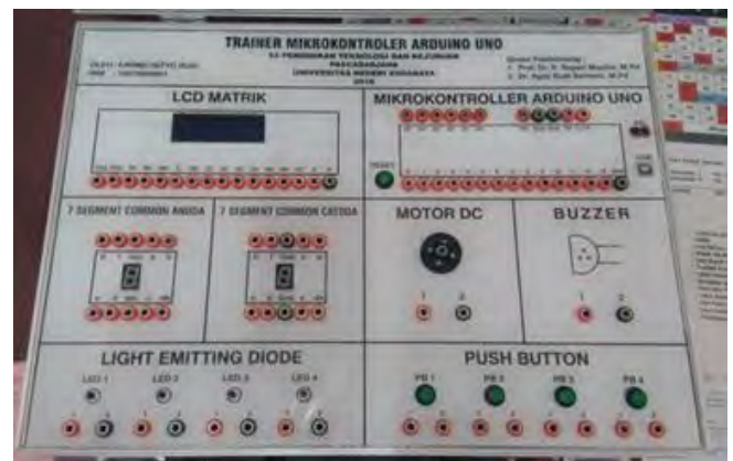
Fig. 3. Arduino based microcontroller trainer media.
