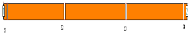
Fig 1.3:- Layout of 0 th order with S_{0,1} = S_{3,4} = 0.437\text{mm} and S_{1,2} = S_{2,3} = 0.801\text{mm}
