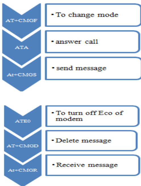
Fig 3.2: Some basic commands of GSM Module
