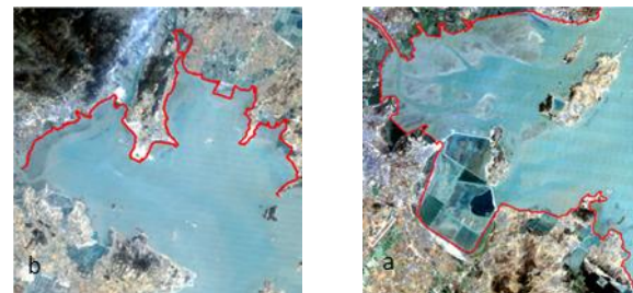
Fig.4. Overlaying of coastline extraction and remote sensing image of Fujian Province's local region a. Fuqing Bay b. Xinghua Bay
