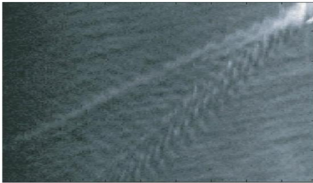
Fig2 SAR image which show ship trail waves
