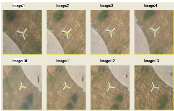
Figure 11. The Adjustment of the GCP
