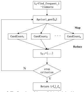
Figure 2. The flow chart of the parallel Apriori algorithm
